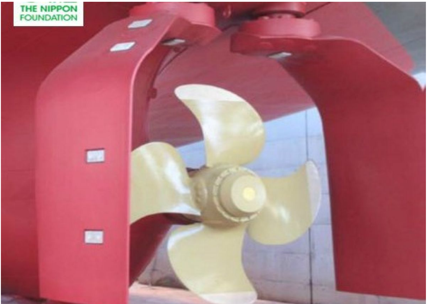
The Gate Rudder system is an example of an Open Type Ducted Propeller.
