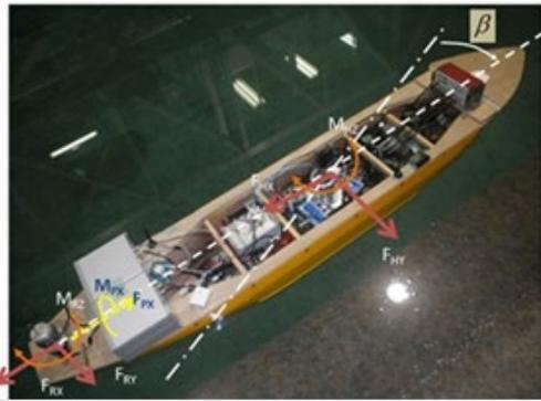
**Photo 3 Test Set up for Rudder Force and Hull Force Measurements**
