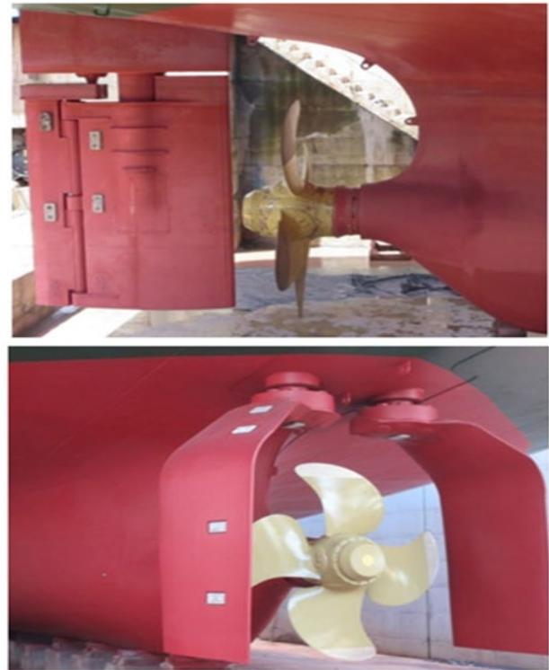
**Photo 1. Conventional Flap Rudder (upper) vs. Gate Rudder(lower)**
