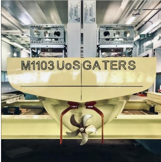
Figure 2 Rudder load measurement system.
