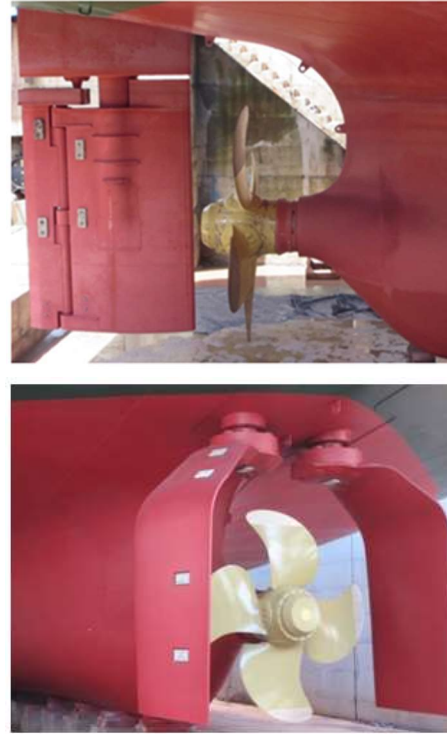
Figure 1. Conventional Flap-Rudder (Top) vs. GATE RUDDER® (Bottom)
