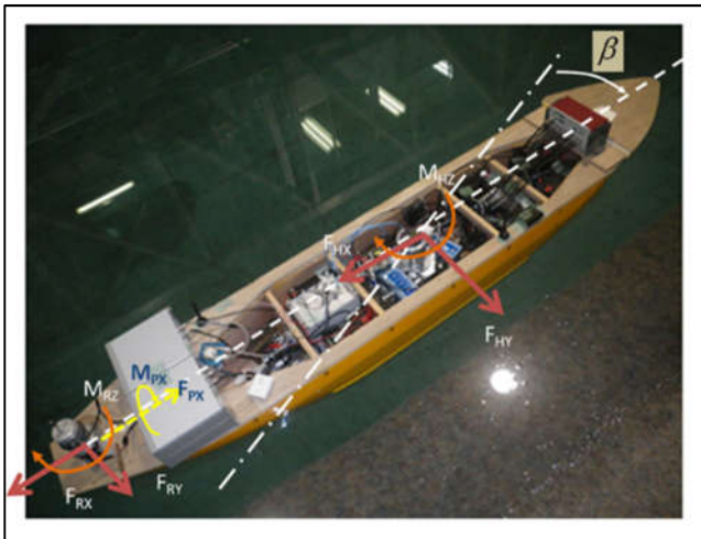
Figure 14. Setup of the manoeuvring test
