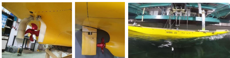
Fig 8. Japanese container vessels (Shigenobu and Sakura) 5m model rudder set up (left) and self-propulsion tests underway (right) at ITU towing tank.
