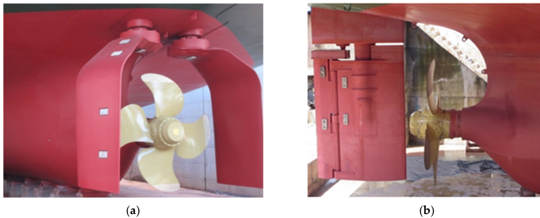
Figure 1. (a) Gate rudder system (GRS) on coastal container ship “Shigenobu.” and (b) conventional flap-rudder system (CRS) on sister container ship “Sakura.”.
