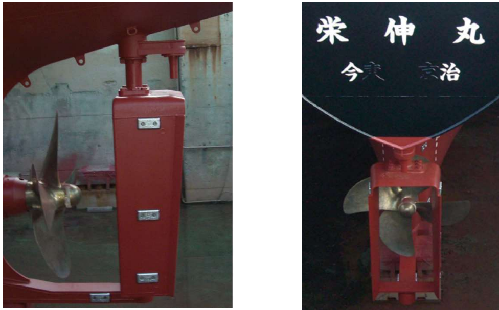
Fig.17 - Installation of Frame Rudder on domestic cargo ship (March 2011)
