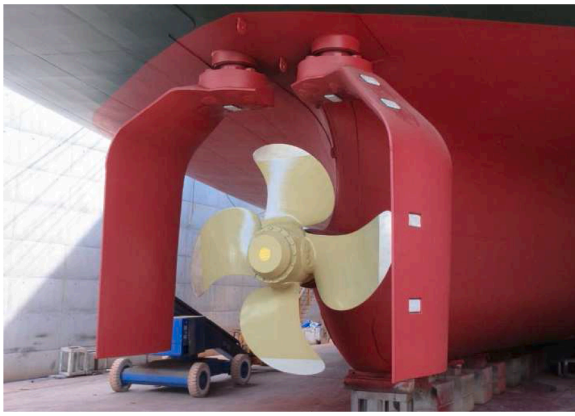
Figure 1. The first application of a Gate Rudder system
