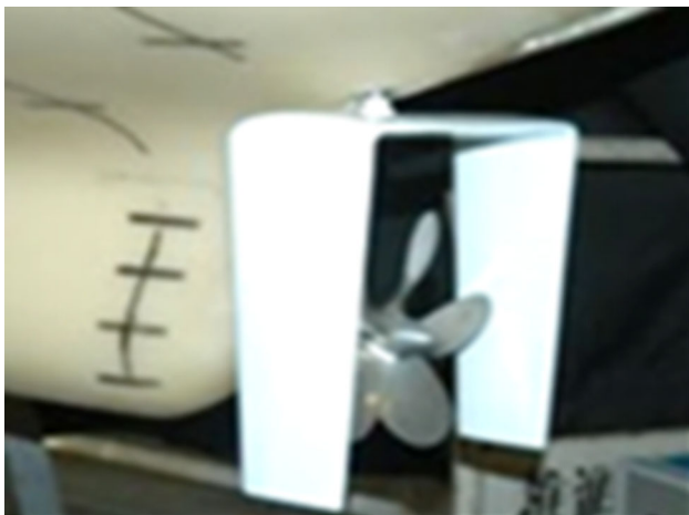
Fig. 3 Model gate rudder fitted to ship model
