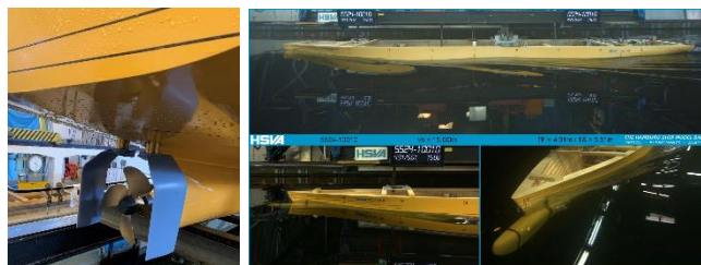
Fig 9. 11m ERGE model GRS set up (left) and self-propulsion tests underway (right) at HSVA towing tank.
