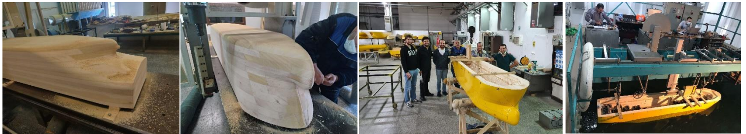
Fig 5 – Physical model (3.6m) manufacture of MV ERGE and resistance tests underway in ITU Ata Nutku Towing Tank
