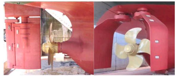
Figure 24. Steering systems of the Sakura (left) and Shigenobu (right).
