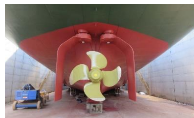
Fig 1 – SHIGENOBU with world's first Gate Rudder System
